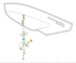
Feed the wires through the cable grommet and assemble the Bracket • with Bracket •.
